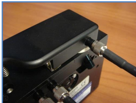
Figure 9: Fiber-optic attached to the top of the CI-710 for Absorbance and Transmittance mode.
