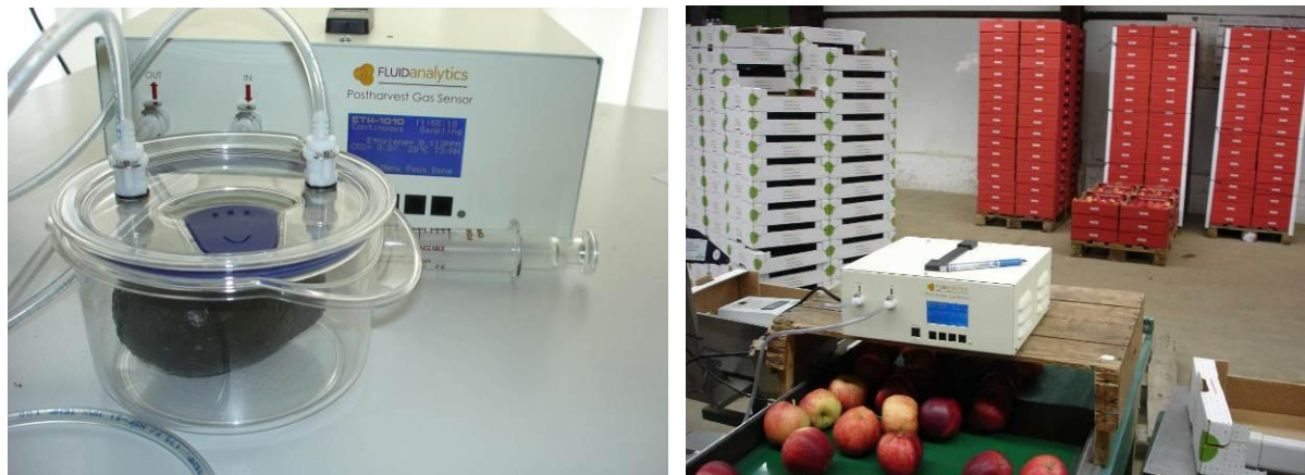
Fig. 5: Left: Closed gas circuit employed to measure real-time continuous ethylene efflux from fruit like avocado; the postharvest gas sensor displays all four, ethylene, CO 2 , temperature and humidity; Right: Continuous in situ measurement in a grading facility with the sorting lines.
