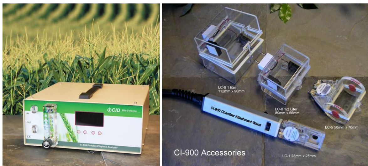
Fig. 3: The ethylene analyser sold under the trademark CI-900 by CID Bioscience (LEFT) Fruit or leaf chamber can be attached to the device for field measurements of ethylene (RIGHT); www.cid-inc.com .
