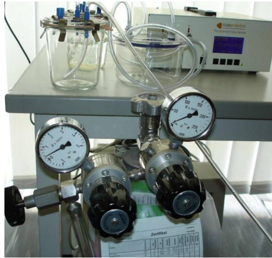
Fig. 4: Calibration setup, which may consist of the standard calibration bottle or the calibration setup provided by the manufacturer (ABSOGES SAS and supplier CID Bioscience).
