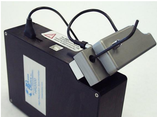
Figure 7: Front View of Leaf Probe connected to Spectrometer.
