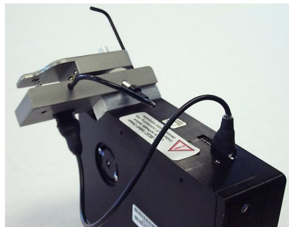
Figure 8: Rear View of Leaf Probe connected to Spectrometer.
