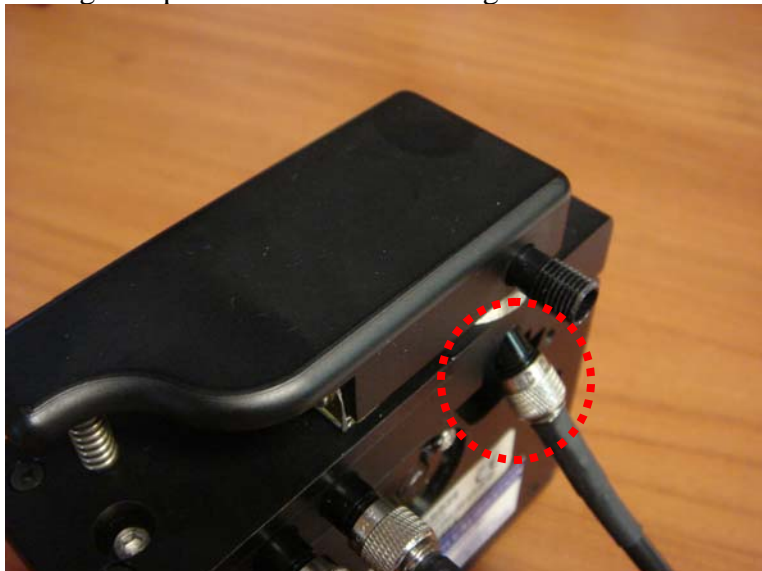
Figure 8. Connecting the fiber optic cable to the lower sampling port for reflectivity measurements
