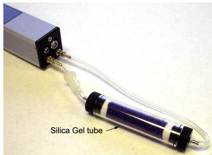
Figure 5-3. Configuration using Silica Gel for H 2 O calibration.
